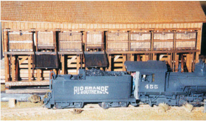
Above right. Richard Marcus, from Staten Island, New York, scratchbuilt an enclosed bucket coaling station from wood. The only commercial parts are the cast metal winch hardware, tools, and figures.
